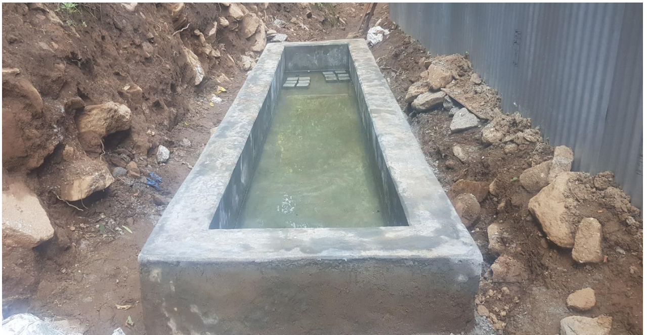
Figure 8: Cube curing pond at concrete lab.
