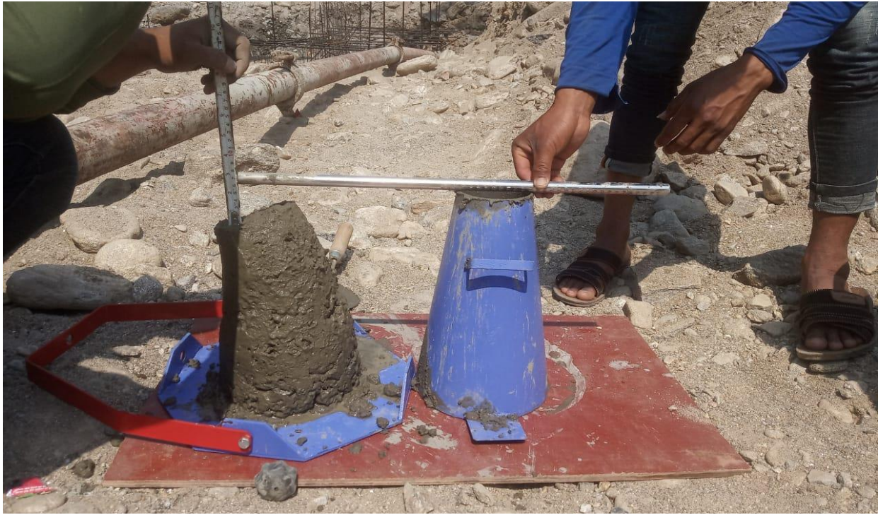
Figure 6: Slump test for in-site quality control.
